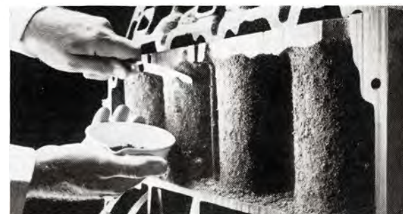
If left unchecked, rust coating on cylinder walls can clog water passages.
